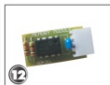
12 Backup Memory Module Back up all the transmitters and operating details set up in the controller
